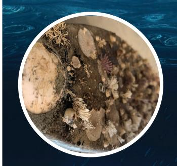
"As fouling grows on the face of a transducer, the amount of detail that you see is significantly reduced."
